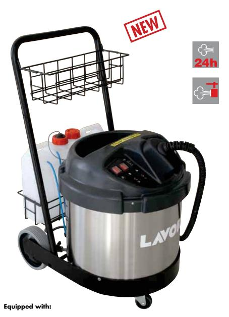
• Satured steam at 9 bar at a temperature of 175°C • Steam gun with low tension control • S/S body AISI 304 • Boiler 3,3 kW S/S AISI 304. Thickness 25/10 • Low level water lamp indicator • Device for using chemicals and detergents mixed with steam • Heating and activation time required: 7 min. • Steam regulation • Discharge valve • Pressure gauge • The boiler can be refilled from the tank provided (continuous duty) • Wheels suitable for food and processing areas • Storage basket
